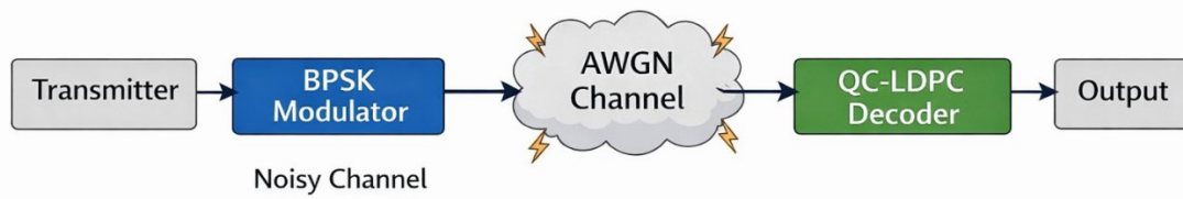
Figure 2. Block diagram of the communication system with QC-LDPC decoding over an AWGN channel.
